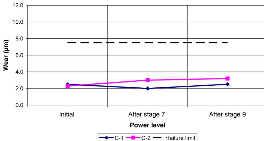
**Graph 3:** Stage by stage breakdown of the wear from BTGS on C-1 and C-2.
