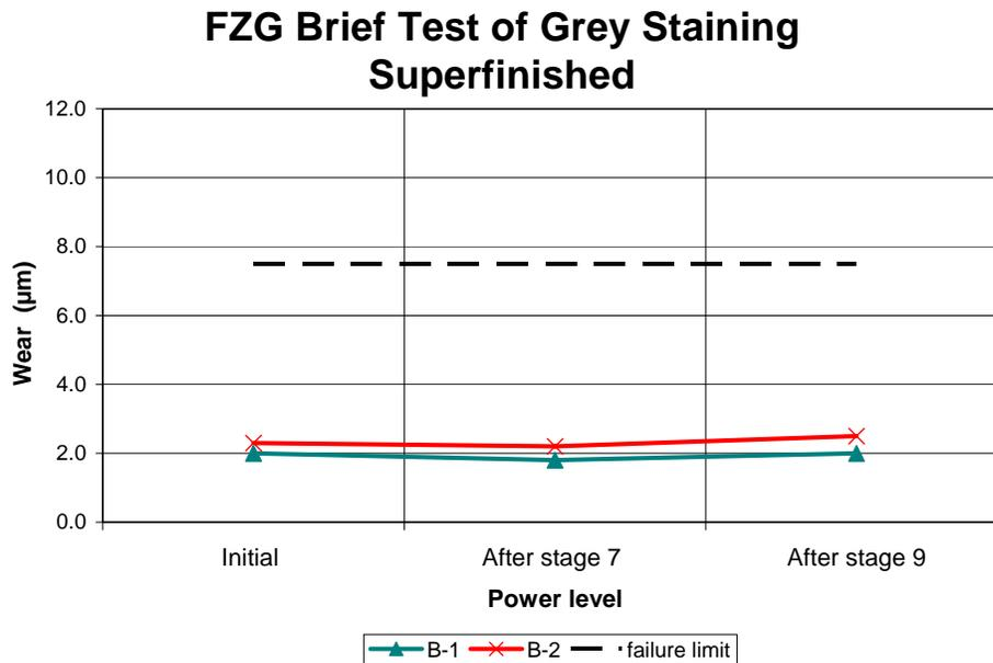
**Graph 2:** Stage by stage breakdown of the wear from BTGS on B-1 and B-2.
