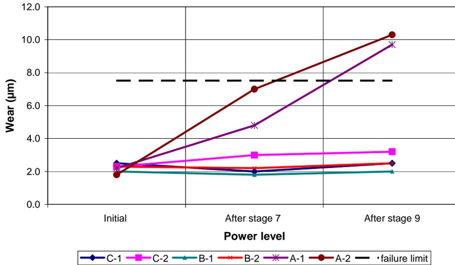
**Graph 4:** Wear summary. A-1 and A-2 are baseline while B-1, B-2, C-1 and C-2 were superfinished. The failure limit is defined at 7.5µm.
