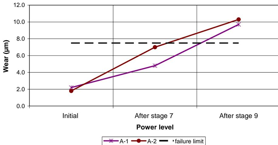
**Graph 1:** Stage by stage breakdown of the wear from BTGS on A-1 and A-2.
